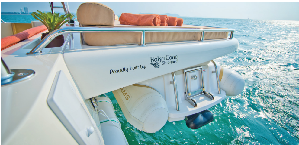
Stern platform with tender protected from weathering
